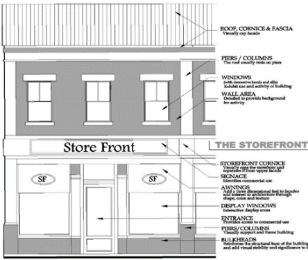
Example of Full Architectural Façade
